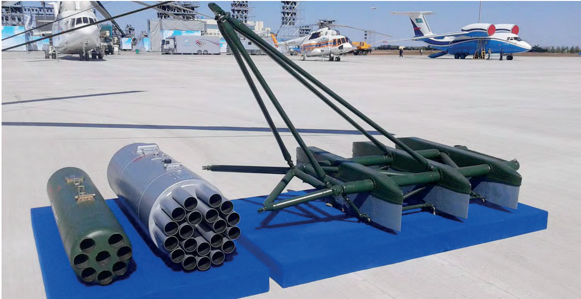
B8V8MSB, B8V20MSB rocket pods and armament rack adapter with BD3-KrV-MSB external store racks designed and manufactured by Motor Sich
